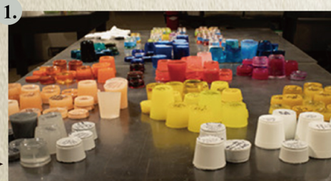
Resin Color Samples 2013-2021. In 2013, I started experimenting with pigmented resin to see what kind of color palette was possible. I still make these color samples today as I'm casting. As you can see, the samples have information written on them, so I can replicate the color ratios when needed.
